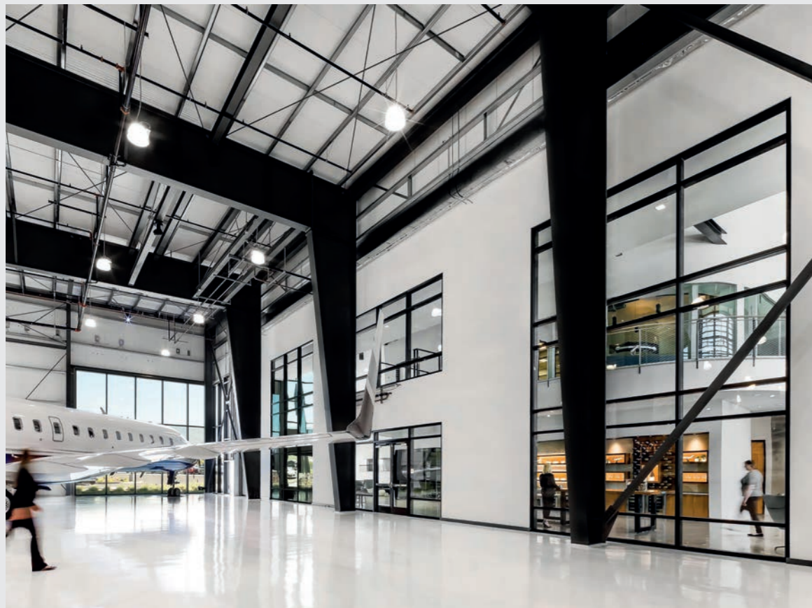
ACI Jet Center, San Luis Obispo (CA), USA Fire-resistant doors – forster fuego light 120 min. (UL10C) – VDS Fire-resistant glazing – forster fuego light and thermfix vario 120 min. (UL263) – VDS Image: Eric Reed
